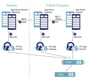
Image above shows the overall tokenization architecture
